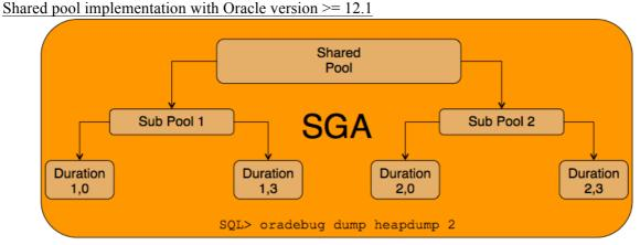
The shared pool structure has changed with Oracle 12.1 once again. Changes for unpublished bug #8857940 are included in 12.1.0.1 and permit to group the shared pool durations in 2 groups, which should allow better shareability of the memory and should avoid unnecessary ORA-4031 errors (MOS ID #1675470.1).
