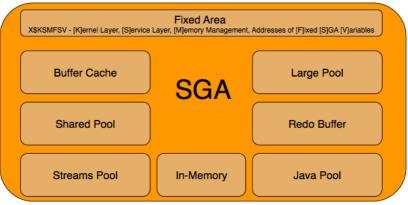
The SGA consists of various components like the "fixed size area", the "variable size area" (java pool, large pool, shared pool, streams pool), the buffer cache (which is also part of the "variable size area" from the OS perspective), the redo buffer and the in-memory area.
