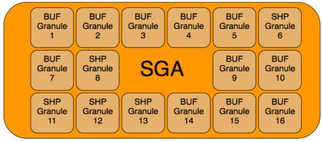
Oracle has re-engineered the SGA in Oracle 9i to move memory between various memory areas like the shared pool, buffer cache, java pool, streams pool and large pool in an easy and "standardized" way. The memory could be moved manually between the key areas in Oracle 9i and starting with Oracle 10g it could be done automatically by the instance itself.
